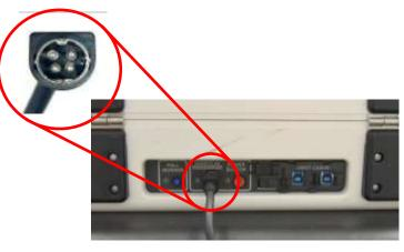
Round end of Power Cable inserted into the back of the Duo
