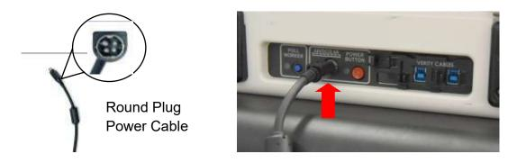
The Round Plug Power Cable has a sleeve that must be slid back to unlock the connection whenever the power cable is unplugged from the Duo.
