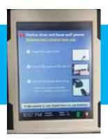
If one or more Duo screens show a red indicator with a line through it on the bottom of the tablet, there is no wall power being supplied to the machine. Trouble-shooting must occur to help correct the problem.
