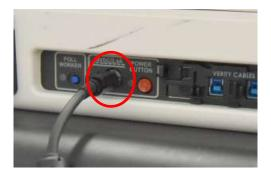
8. Connect the Verity Data Cable coming from the Duo on the accessible booth located closest to the Controller, into one blue port on the back of the Controller.
