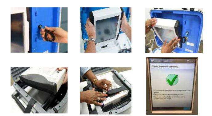
7. Once the Duo tablet is connected and secured in the Duo Go, insert Ballot Paper into the black Duo Go printer marked "Brother." The ballot paper arrow will be facing the printer slot. When the paper is inserted correctly there will be a green check mark. Follow the instructions on the tablet screen.
