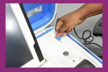
11. Press the Red Button on the back of the Controller to power it on.
