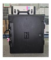
2. Reach inside the Ballot Box and pull the white string down and away from yourself to lock the Scan. Gently lift the handle of the Scan to confirm it is locked in place.
