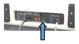
Slide open the dust cover and plug the ATI into the Duo here.
