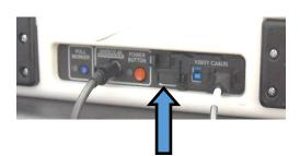
Slide open the dust cover and plug the ATI into the Duo here.
