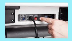
Wait for the Controller to completely power down and display a black screen before starting to take down the Controller.
