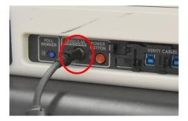
8. Connect the Verity Data Cable from the Duo on the accessible booth, located closest to the Controller, into one blue port on the back of the Controller.
