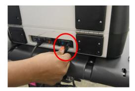
Never tilt the Controller, Duo, or Scan by the handle when cables are connected. This can damage the cables where they connect or cause damage to the device itself.
