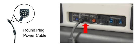
The Round Plug Power Cable has a sleeve that must be slid back to unlock the connection whenever the power cable is unplugged from the Duo.
