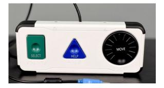
A Voter may plug their sip-and -puff, tactile switches, or other dual-switch input devices into the appropriate port on the top of the ATI.
