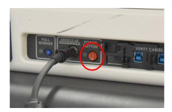
The power-on process for the Duos, Controllers, and Scans takes 4 ½ minutes for each machine. Do not be alarmed when the screen does not turn on immediately and goes dark twice during the power on self test.
