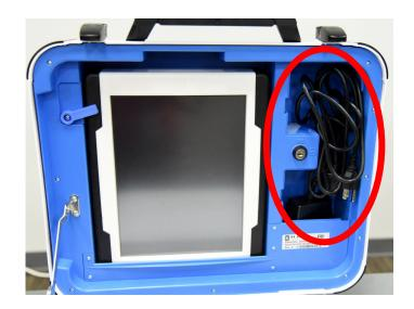
7. Connect the two parts of the power cord, then connect the cord to the back of the Controller using the round power plug. The flat side of the plug faces up.
