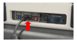
The Round Plug Power Cable has a sleeve that must be slid back to unlock the connection whenever the power cable is unplugged from the Duo.
