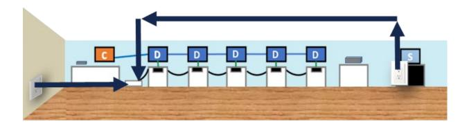
Extension cords are used to help supplement outlet access where needed. All cords must be out of the path of Voter traffic. No mats can be used to cover cords under any circumstances. For help in identifying solutions to connecting equipment to power during the setup process call 713-755-1617, Option 4.
